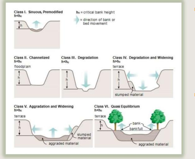
All alluvial streams respond in the same gravity-driven process to any form of hydromodification (landscape or in-channel), as described by Simon's (1989) model of channel response in disturbed alluvial channels
