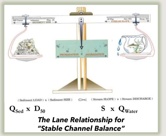
Alluvial streams and their floodplains form in a "dynamic equilibrium" balance to do the work of moving water and sediments through the system most efficiently in response to watershed hydrology and sediment loads
